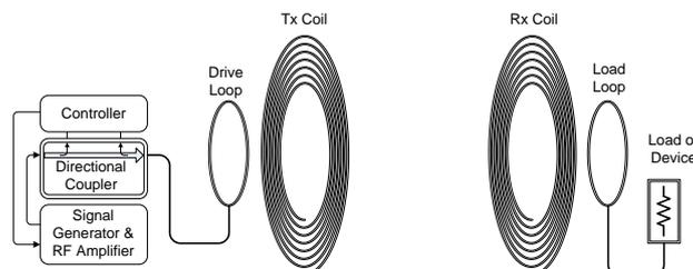
Figure 1: Schematic block diagram of magnetically coupled resonant wireless power system. A two element transmitter, comprising a loop and high-Q coil wirelessly powers a similar two element receiver. Reprinted from [3], ©IEEE.
